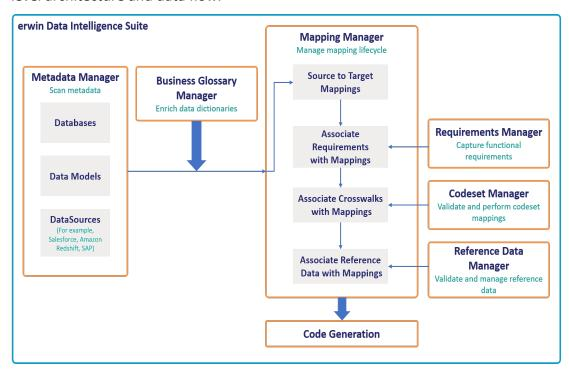
The following sequence gives a high-level understanding of how the modules interact in a typical data integration project:
